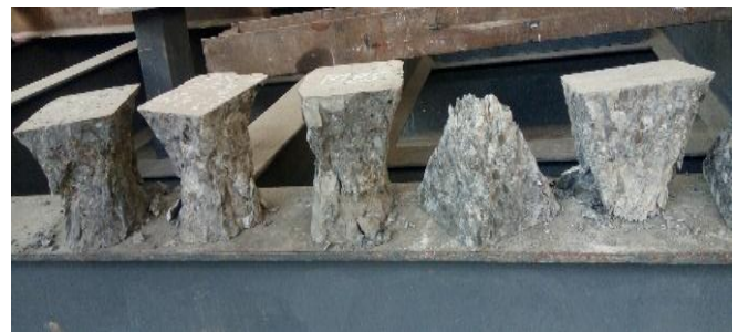
Fig-4: Break behavior of tested cubes.
