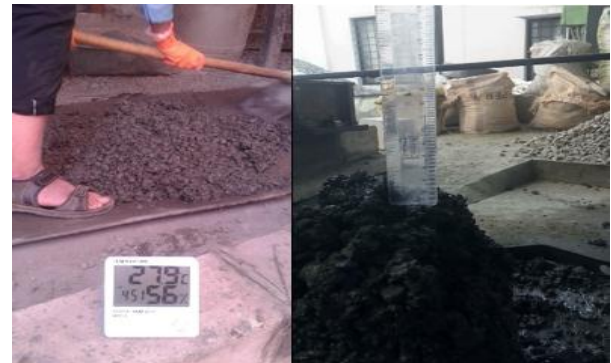
Fig - 2: Slump test
