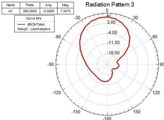
Fig 3. Simulated 2X1 microstrip patch antenna Directivity
