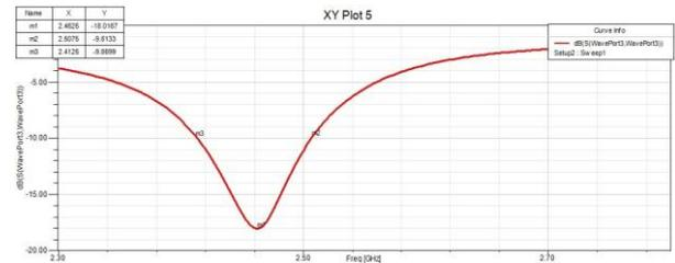
Fig 8. Simulated 2X1 microstrip patch antenna S11
