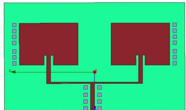
Fig 2. Simulated 2X1 microstrip patch antenna design with EBG
