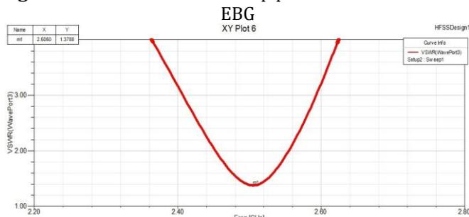
Fig11 . Simulated 2X1 microstrip patch antenna VSWR with EBG
