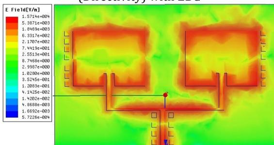
Fig 13. Simulated 2X1 microstrip patch antenna Current with EBG
