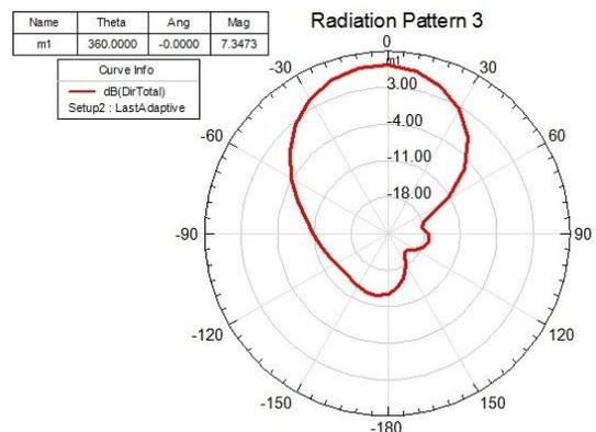
Fig 9. Simulated 2X1 microstrip patch antenna Directivity with EBG
