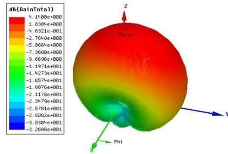
Fig 6. Simulated 2X1 microstrip patch antenna GAIN 3D (Directivity)
