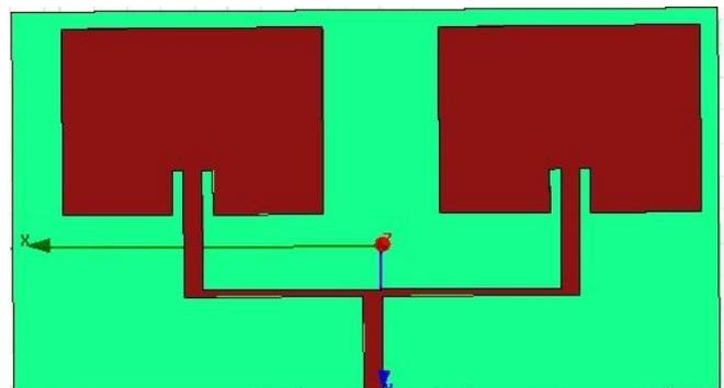
Fig1. Simulated 2X1 microstrip patch antenna design
