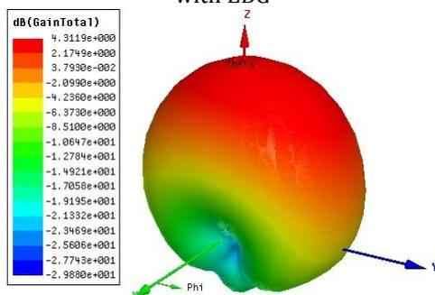
Fig 12. Simulated 2X1 microstrip patch antenna GAIN 3D (Directivity) with EBG
