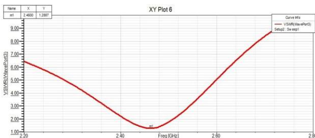
Fig 5. Simulated 2X1 microstrip patch antenna VSWR
