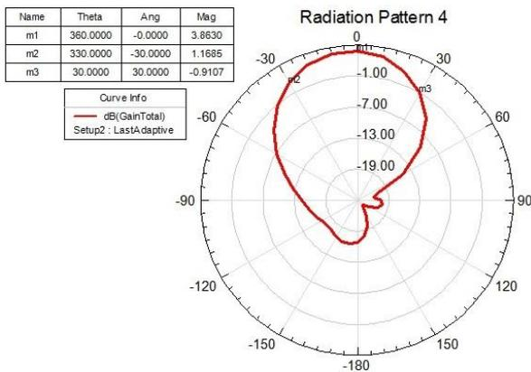
Fig 4. Simulated 2X1 microstrip patch antenna Gain
