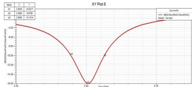
Fig 14. Simulated 2X1 microstrip patch antenna S11 with EBG
