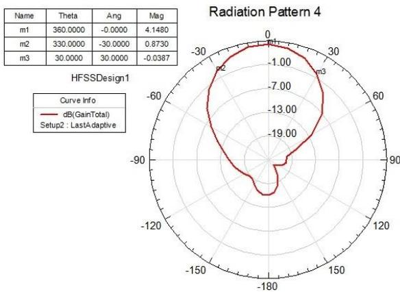
Fig 10. Simulated 2X1 microstrip patch antenna Gain with EBG
