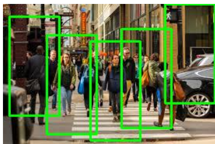
Fig. 3. Result of Non Maximum Suppression for the first test image
