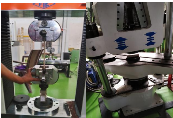
Fig.8 Strip loaded on UTM machine for Tensile and compressive testing.
