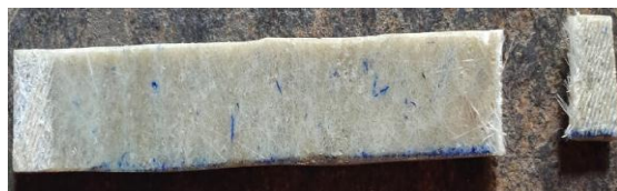
Fig.7 GFRP material strip after tensile testing.
