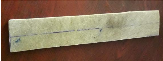
Fig.6 GFRP material strip before tensile testing
