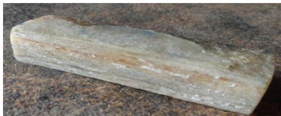
Fig.8: GFRP Specimen for compressive testing
