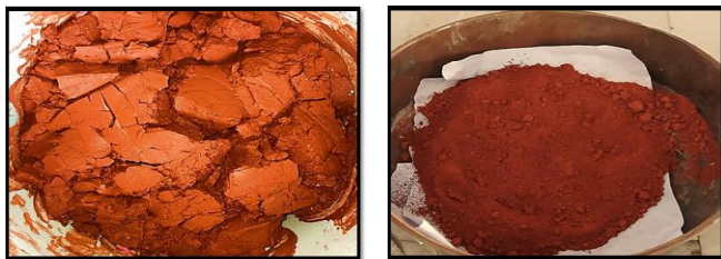
(a) Wet Red Mud collected from Damanjodi, Koraput Odisha, India (b) Oven Dried Red Mud
