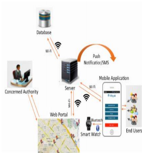
Fig- 2: Smart mobile based emergency management architecture
