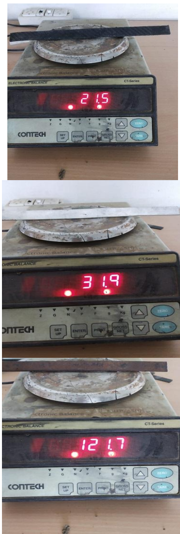
Fig -1: Weight of Carbon Fiber vs. aluminium and Steel. B) Tensile Strength of Carbon Fiber vs. Aluminium and Steel
