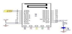
JDY-31 Bluetooth is based on Bluetooth 3.0 SPP design, which can support Windows, Linux, android data transmission, working frequency band 2.4GHZ, modulation mode GFSK, maximum transmission power 8db, maximum transmission distance 30 meters, support users to modify device name through AT command The baud rate and other instructions are convenient and quick to use.
