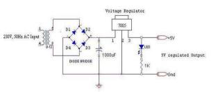
Regulated power supply is the main component of electrical, electronics and as well as automation equipment. Mobile phone charger, oscillator, amplifier are needed the regulated power supply.
