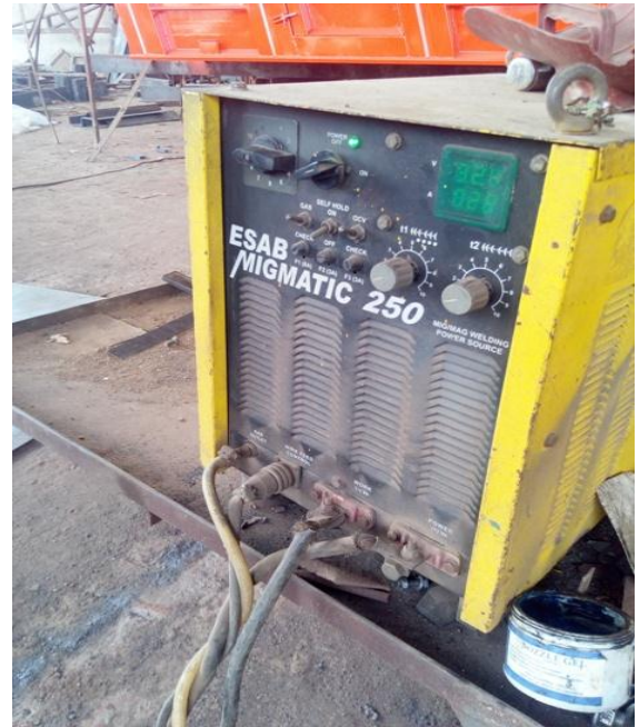
Figure3: ESAB MIGMATIC 250 MIG welding machine
