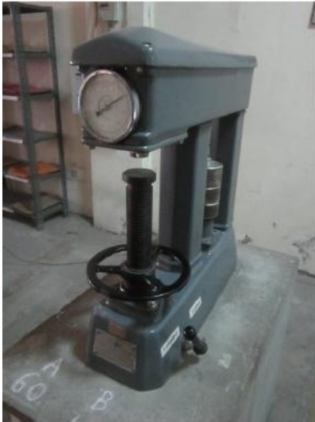
Figure 5 Rockwell Hardness Tester for measuring specimen hardness
