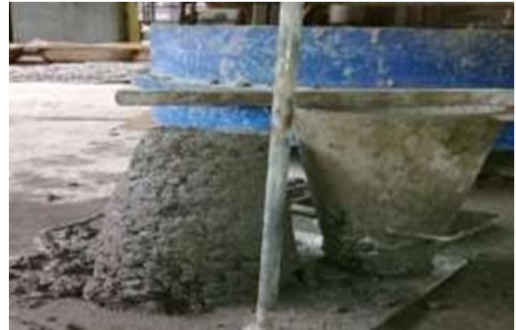
Fig. 2: Workability Test Conducted in Lab
