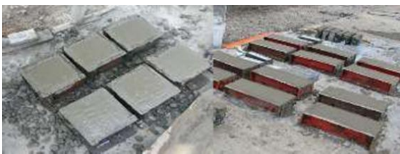
Fig. 1: Casting of Cubes, Beams, and Cylinders
