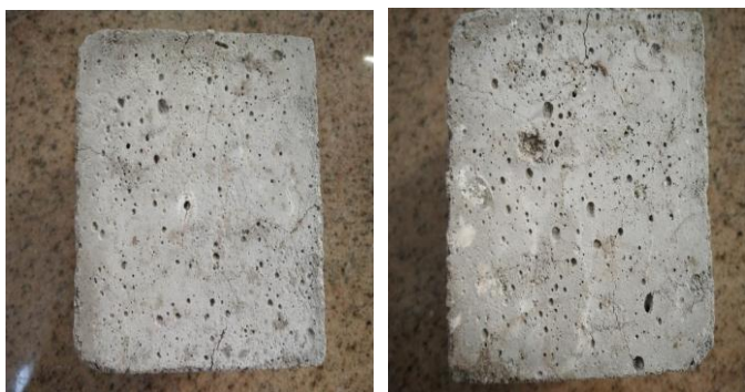
Fig 10 and 11: Concrete specimens subjected to 400°C and 600°C
