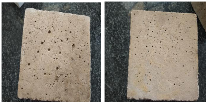
Fig 8 and 9: Concrete specimens at room temperature and subjected to 200°C
