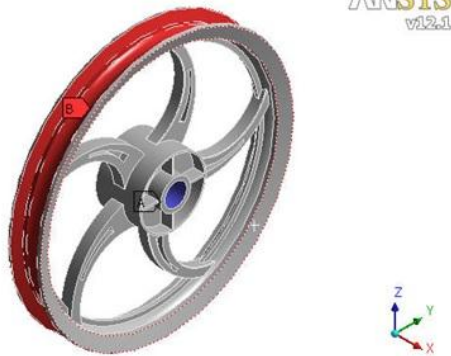
Fig 5: Boundary Condition with Pressure
