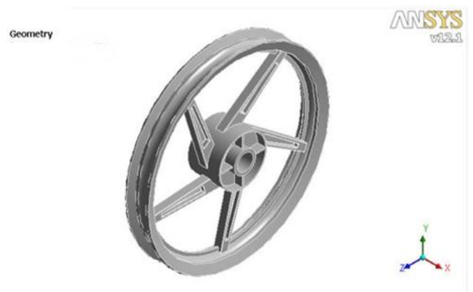
Fig 3: ISOMETRIC VIEW OF WHEEL RIM MODEL 2 (inclined spokes)
