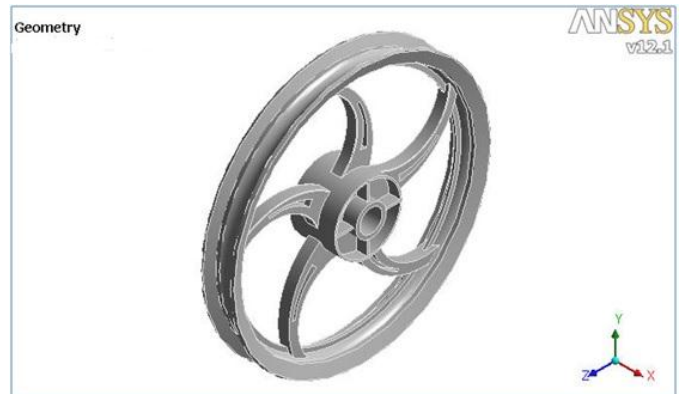
Fig 2: ISOMETRIC VIEW OF WHEEL RIM MODEL 1 (curved spokes)
