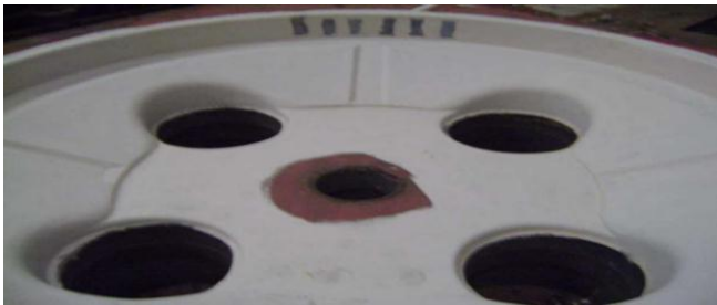
Figure 3.5 Mould cavity of Bowl including 4 risers
