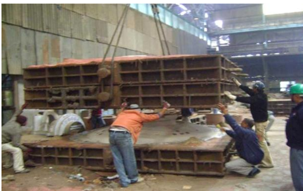
Figure 3.7 mould closing of Bowl
