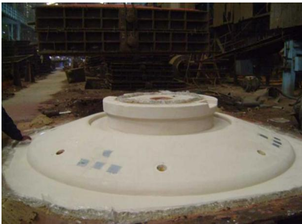
Figure 3.6 Core Setting of core no.2
