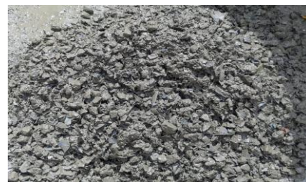
Fig-1 waste Tyre rubber pieces added to Concrete
