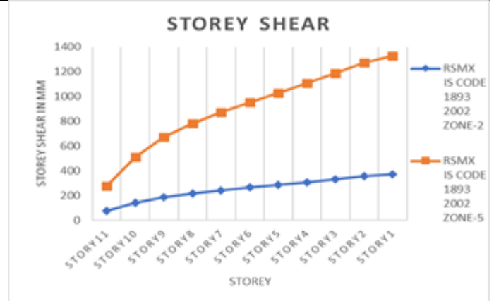
Fig-17 Storey Shear of Model in Z- II and Z-V subjected to RSM.
