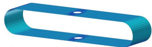
Fig -1: Shell model of the Isolator
