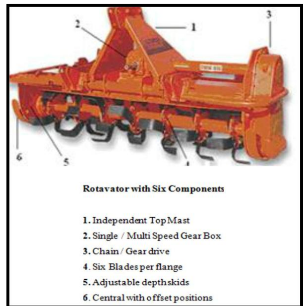
Fig.1 Rotavator with six Components
