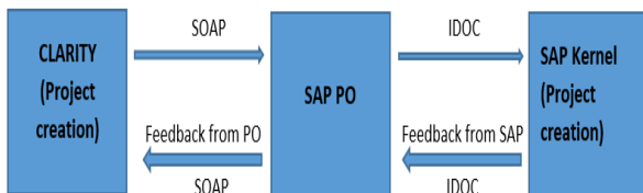
Figure 3: Flow of Project creation from Clarity to SAP using SAP PO
