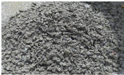
Fig-1 Crushed Coconut Shell added to Concrete
