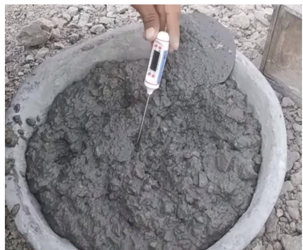
Figure7- ASTM C064 Standard Test
