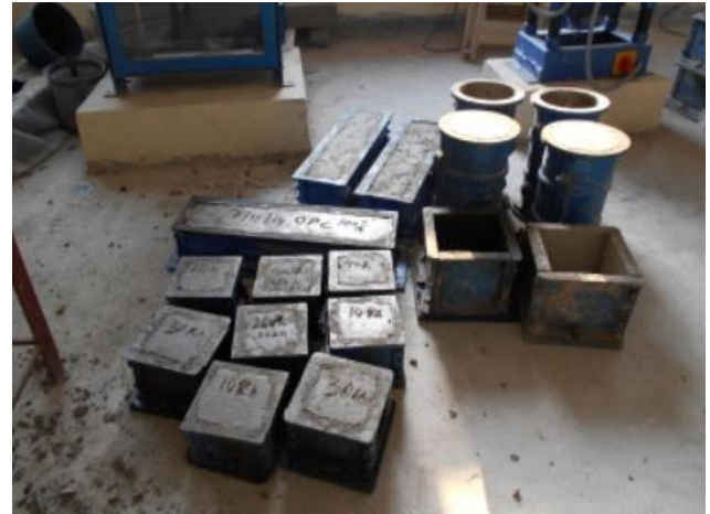
Figure1- Casting of Specimens
