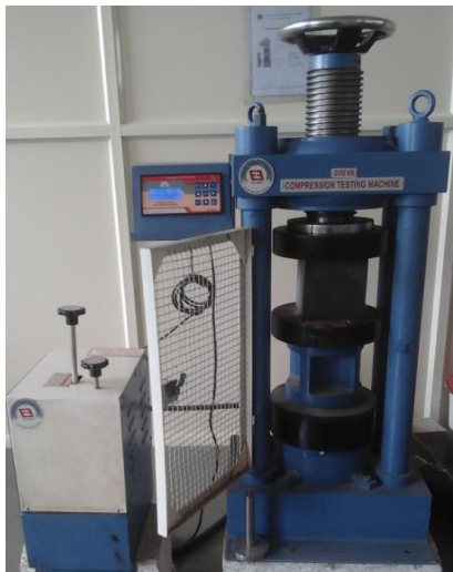
Figure8-Testing of Cube for compression test
