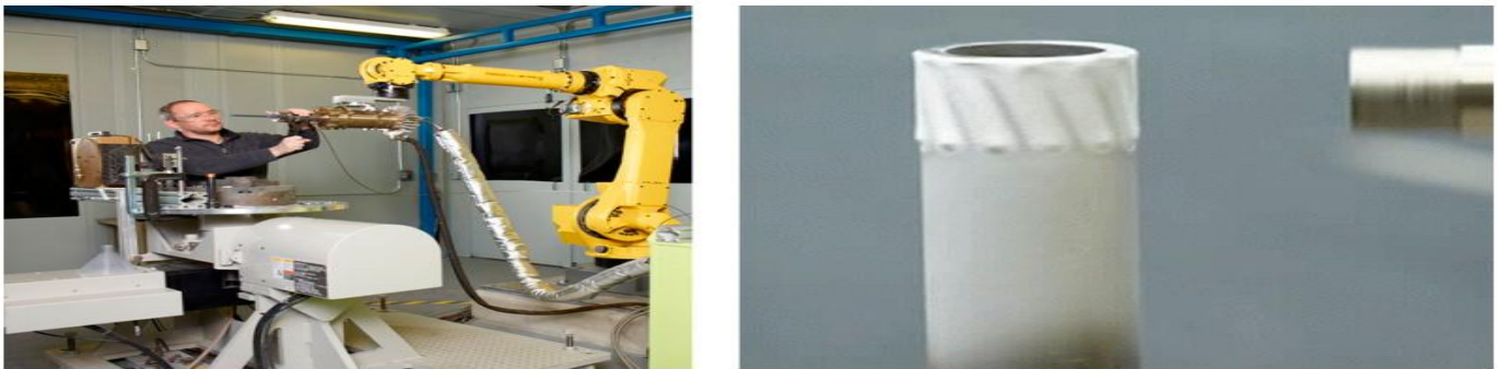
Fig8: (Left) Operator setting up cold spray AM system, which operates outside of a controlled environment and (right) cold spray deposit forming on the tip of a substrate tube that is rotated
