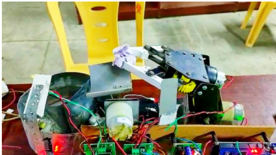
Fig-2: After picking the waste the arm place it on the collector unit.
