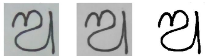
Fig-3: (a) RGB image (b) Grayscale image (c) Threshold binary image
