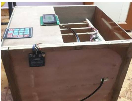
Fig. 11 External view showing LCD, Keypad, RFID reader
