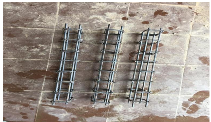
Fig -3.2: reinforcement cage
