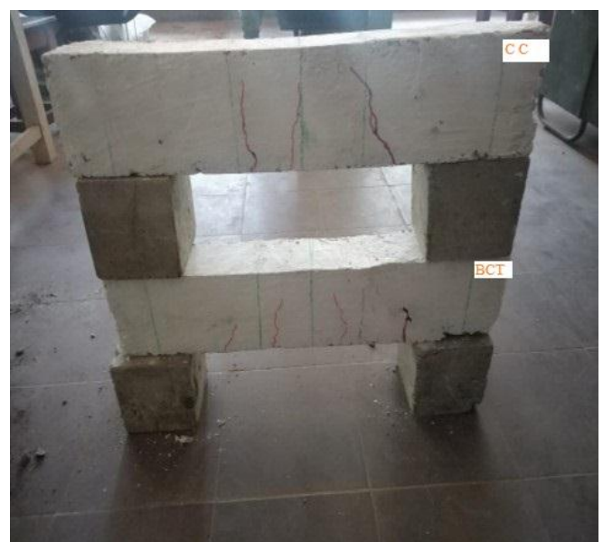
Fig -3.3: Crack pattern of flexural specimen
