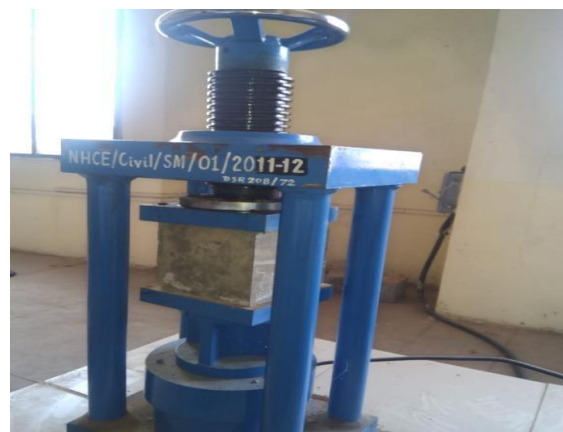
Figure 3.1 Testing of concrete cubes at NHCE Concrete Technology lab.
