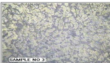
Fig 7: Microstructure of AA2011 with 10%Wt of Flyash
