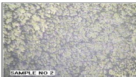
Fig 6 : Microstructure of AA2011 with 5%Wt of fly ash
