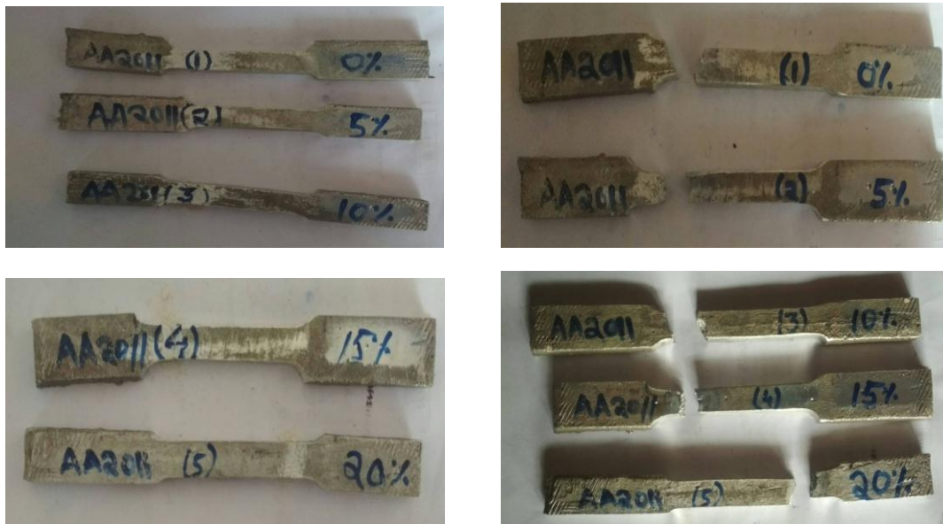
Fig 14: Al Cast Alloy in sync with ASTM E8 Standards
