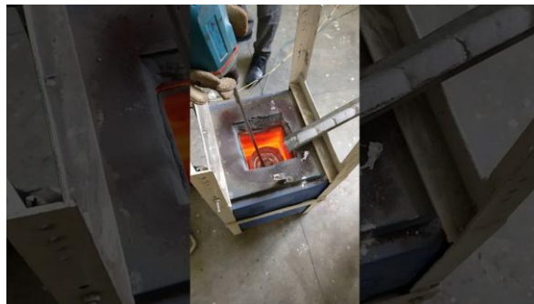
Fig 3 : Stir Casting Process
