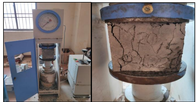
Fig -2: (a) Compressive strength test and (b) Cracked cube after compressive strength test
