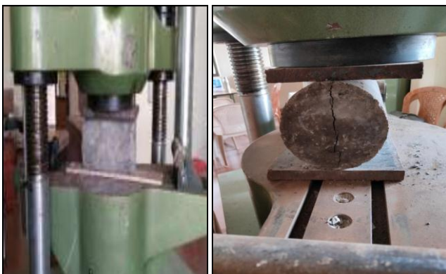
Fig -3: (a) Split tensile strength test and (b) Cracked cylinder after split tensile strength test
