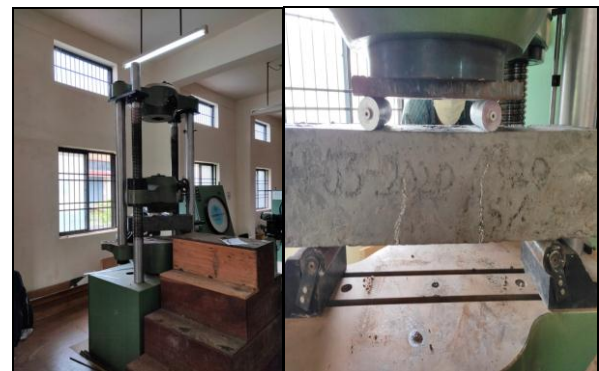
Fig -4: (a) Flexural strength test and (b) Cracked beam during flexural strength test
