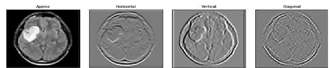
Fig -8: 1 st level DWT Decomposition
