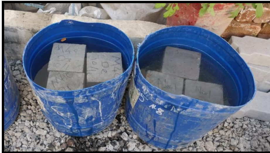
Figure- 3: Water absorption test
