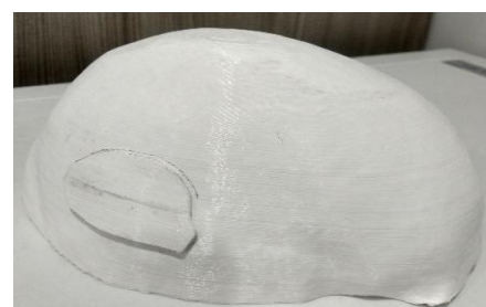
Fig -10 : 3D printed image of Skull with separately made implant glued to the surface
