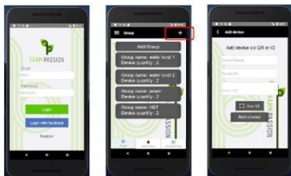
Fig. 3. Android application result (a) log in page (b) add device (c) add device using QR code or sensor ID
