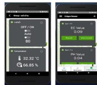
Fig. 4. Individual sensor page on Android application (a) humidity and temperature monitoring (b) EC and pH monitoring.
