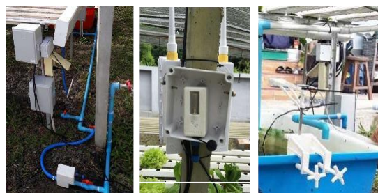
Fig. 2. Sensor installation (a) foggy solenoid valve (b) humidity and temperature sensor (c) water level sensor
