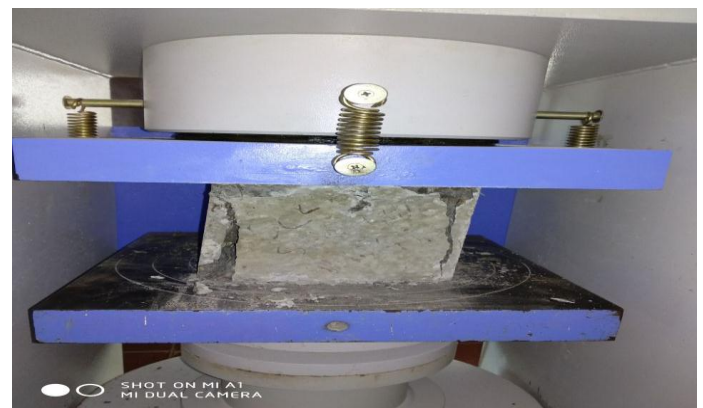
Figure-3: Cube Specimen after failure
