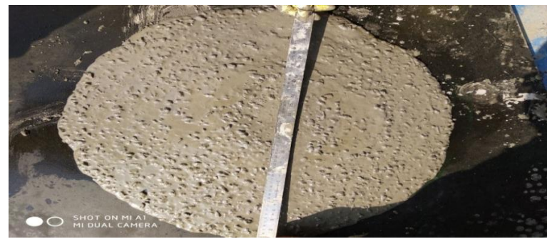
Figure-1: Slump flow test
