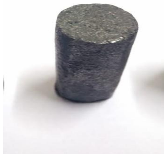
Fig-1 : Samples of brake pad material in cylindrical shape
