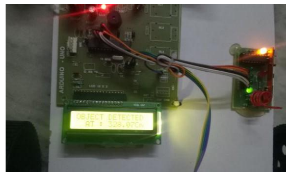
Fig 13. Collision avoidance through Obstacle Detection
