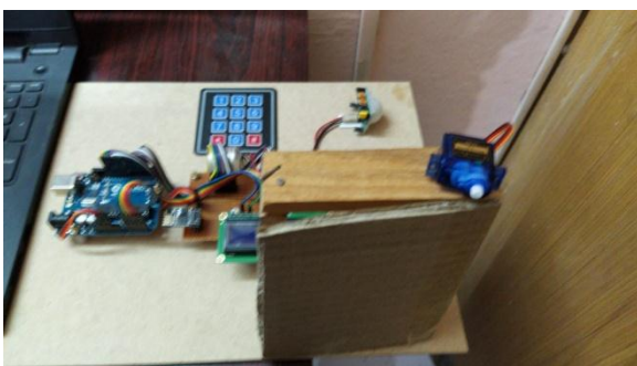
Fig 7.1: Hardware Kit of Door Lock system
