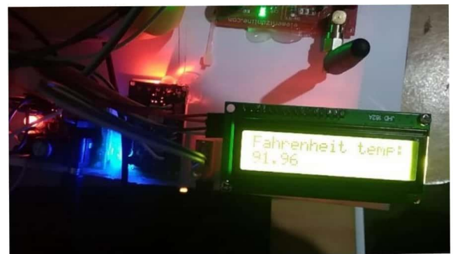
Fig -4.8: Output of the temperature sensor displayed on the LCD screen.
