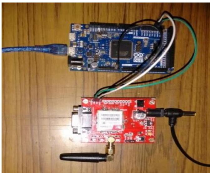
Fig -3.3: GSM module connection with Arduino.
