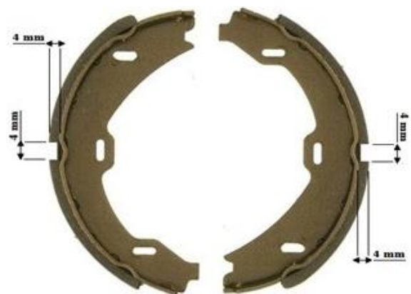
Fig - 5: Modified brake shoe with one slot.
