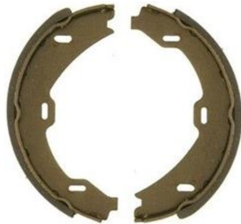
Fig - 4: Plain brake shoe (original without modification).
