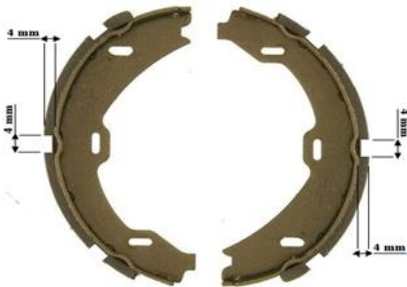
Fig - 6: Modified brake shoe with three slots.
