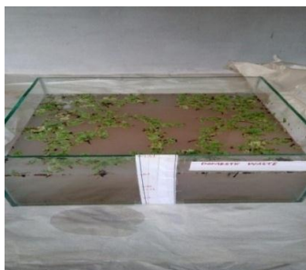
Fig -7: Initial stage of filling azolla in the trough containing domestic wastewater
