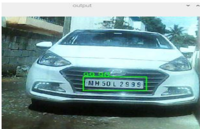
Fig -12: Screenshot of Detected Vehicle Number Plate
