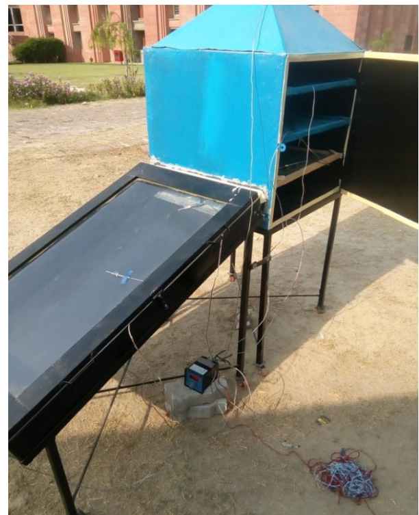
Fig 8 Natural solar dryer in the presence of sun
