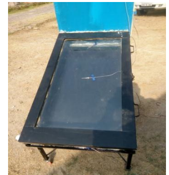
Fig 4 six point thermocouple Fig 5 solar absorber( collector) plate
