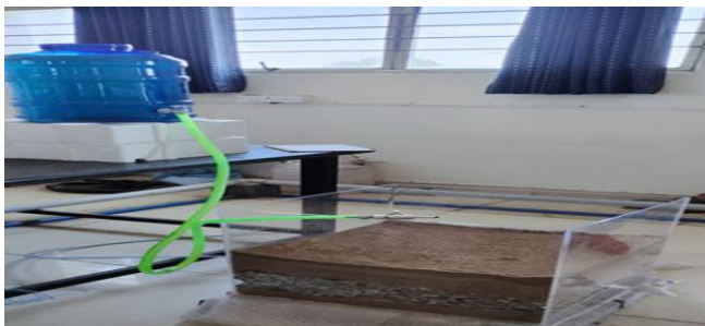
Figure 9.0 Inlet Pipe Valve used for VFCW
