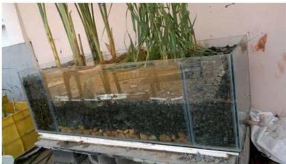
Figure 14.0 Design of Horizontal Flow Constructed Wetland
