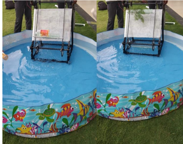
Fig.5: Waste is lifted by the model.
