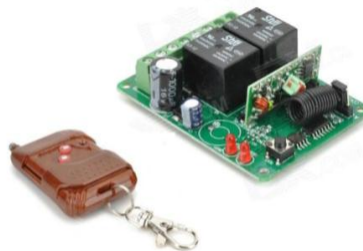
Fig.12 RF Transmitter andReceiver
