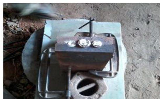
Fig.4 Molten metal in the Mould
