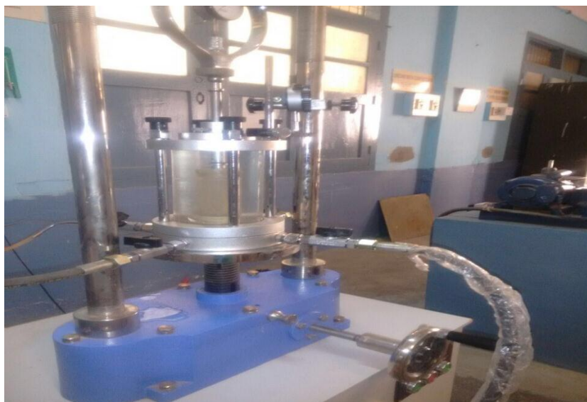
Fig 2 : Triaxial Compression test equipment
