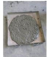
Figure 7. Slump flow ABRAM'S cone
