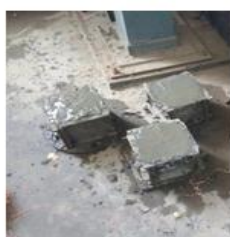
Figure 8. Cube & Cylinder casting
