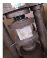
Figure 10. Cube & Cylinder Testing
