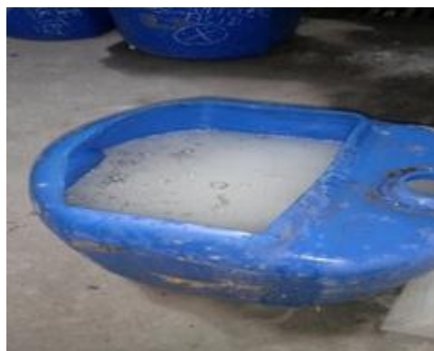
Figure 3. Acid curing barrel (comprising 5% Conc. Sulphuric Acid)
