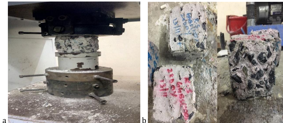
Figure 6. (a) Compressive testing of acid cured cube specimen
