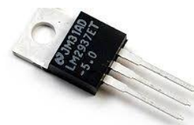
Fig -10: Voltage Regulator
