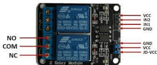
Fig -8: Relay Module
