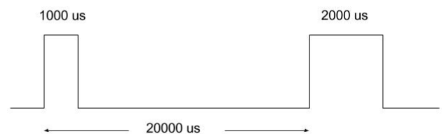
Fig 2.1: Pulse Width Modulated signal.
